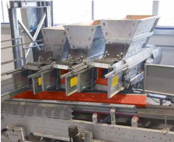
Color-Mix shuttle belt system
